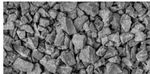
Figure 3 Macadam: compacted layers of broken stone of even size for surfacing roads and paths
