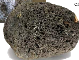
Figure 2 . First lightweight aggregates used in concrete mixtures: pumice (top), tufa stone (middle), and scoria (bottom).
