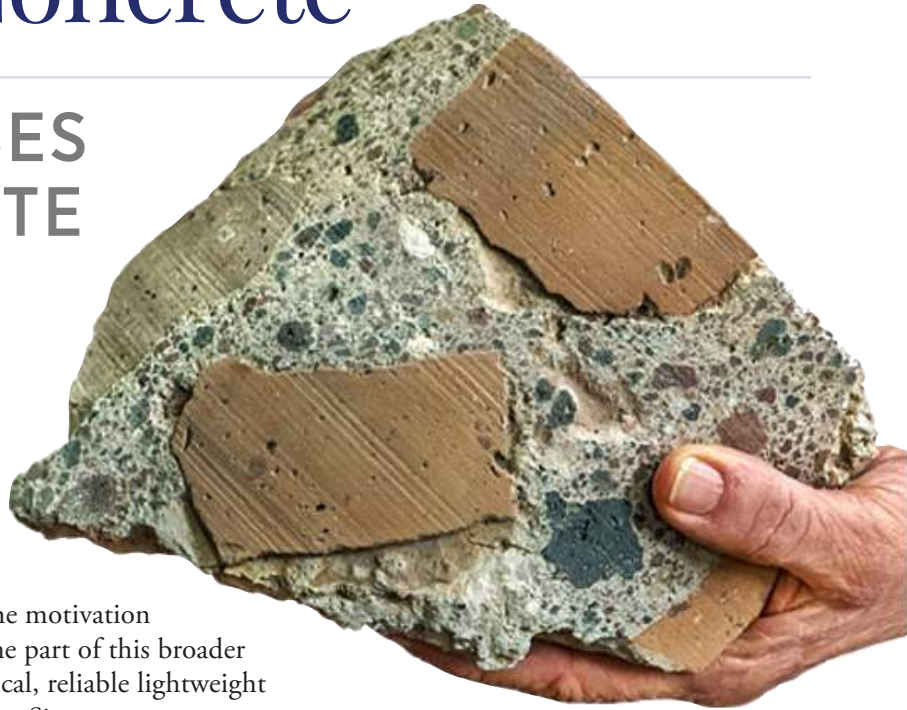
Figure 1 Ancient Roman concrete consisting of chunks of volcanic tuff and brick bound together by a volcanic ash-lime mortar Image: Roy Kaltschmidt, Berkeley Lab
