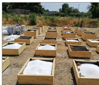
Figure 5 • Construction phase: fine perlite addition in containers.
