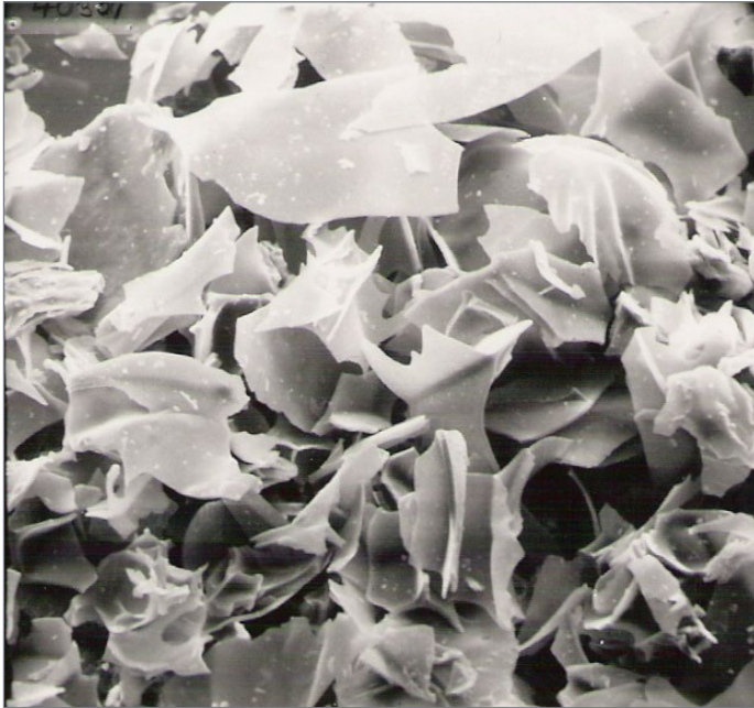
Characteristic structures of expanded perlite flake filler (left) and microspheres (right).
