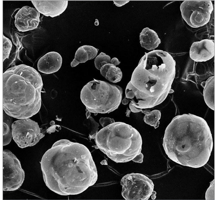
Characteristic structures of expanded perlite flake filler (left) and microspheres (right).
