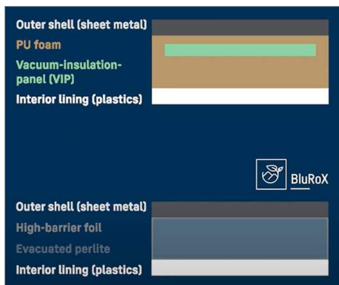
Figure 7 • Traditional design (top) versus the innovative BluRoX freezer wall containing evacuated perlite.
