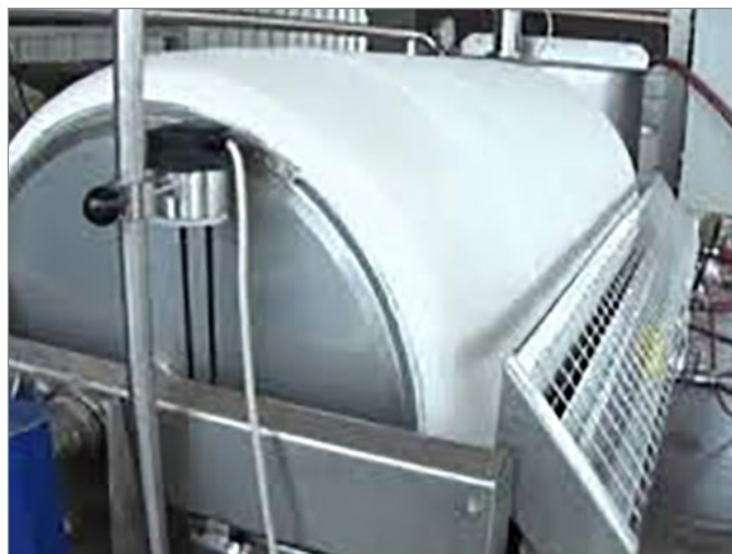
Figure 3 • Drum filter with PFA precoat
