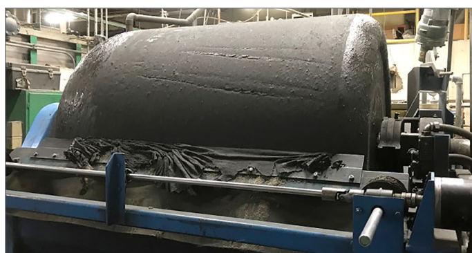
Clockwise from Left: A drum filter septum; adding perlite filter aid to the precoat tank; the septum with perlite precoat; the drum filter during operation.
