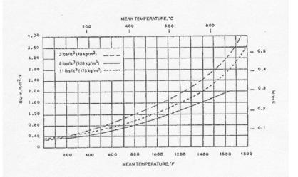
Figure 1 - Thermal conductivity of expanded perlite at three different densities at temperatures from  $100^{\circ}$ F to  $1800^{\circ}$ F (40°C to  $980^{\circ}$ C).
